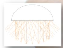
The light outputted by the large emitting area of the Cool Plasma lamp inside our specially designed, highly specular hood, is spread evenly underneath it, instead of coming from a point source, such as with the HPS and HID.
